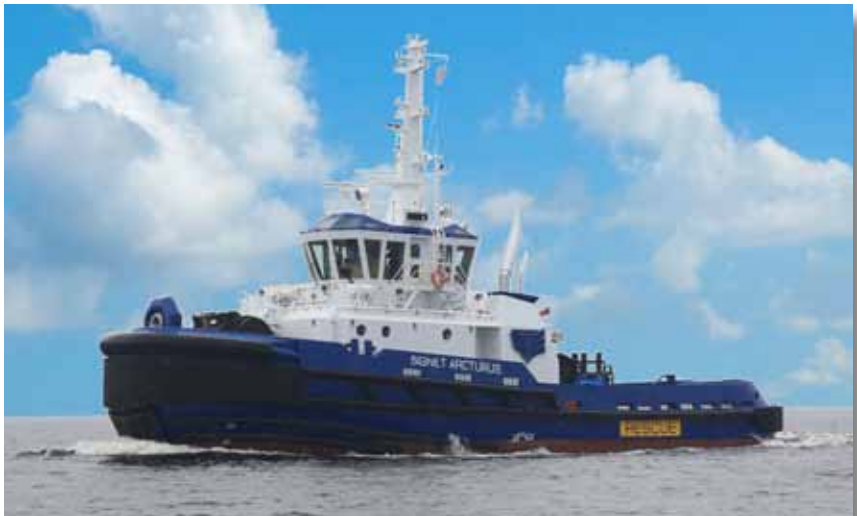
The SIGNET ARCTURUS with its 83.45 metric tonne bollard pull is designed to support offshore towing, rig escort and subsea expansion.
