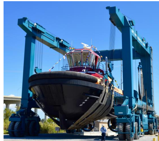
GLADYS B mobilized and launched by 660 ton Travelift at Signet Shipbuilding & Repair
