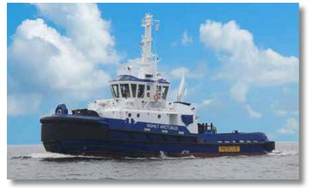
The SIGNET ACTURUS with its 83.45 metric tonne bollard pull is designed to support offshore towing, rig escort and subsea expansion.
